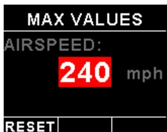
This display can be accessed by pressing the F2/Down button during the normal display mode. Press the F1/Up button when the max values display is showing to reset the maximum values to the current airspeed.
