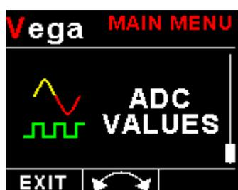
This menu displays the ADC value that have been read from the airspeed pressure sensor.
