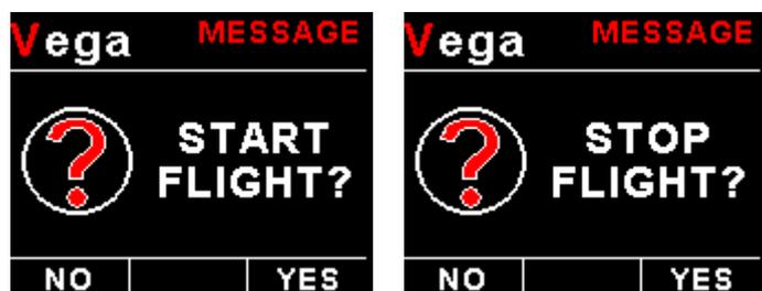
Press the F1/Up button during the normal display mode to manually start/stop a flight. This key is only active if the ASV-1 is setup to select the manual flight option under the "TIMERS" setup menu.
