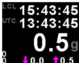
Slip Indicator & OAT disabled, Flight Timer set for remote start/stop
