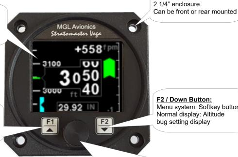
F2 / Down Button: Menu system: Softkey button Normal display: Altitude bug setting display
