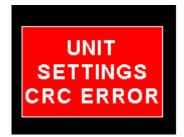
Unit settings CRC error. Load default settings to restore to factory defaults. If the error message still persists then it could possibly be a non-volatile memory failure in which case the instrument will then have to be returned to the factory.
