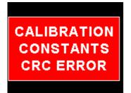
Calibration constants CRC error. The instrument could possibly have a non-volatile memory failure in which case the instrument will then have to be returned to the factory.
