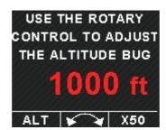
Press the F2/Down button during the altitude "TAPE" display to access the altitude bug setting screen. Press the F1/UP key to set the altitude bug to the current altitude or use the rotary control to adjust the altitude bug. Press the F2/Down key to change the increment / decrement unit to 50 or 500. Press the rotary control to exit and save.
