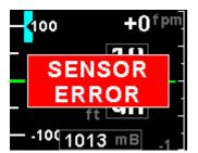
Altitude sensor error. The instrument could have a faulty altitude sensor in which case the instrument will then have to be returned to the factory.
